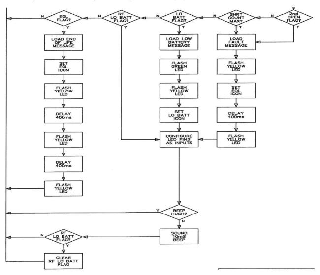
The special state "fault" signals are shown above in the flow chart.
